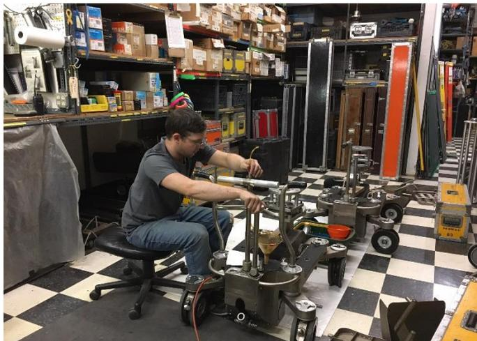
*Picture above: one employee empties the hydraulics on a camera dolly to keep their equipment well maintained.*
